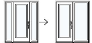
Designed to replace an entrance configuration with 33 $\frac{3}{4}$ " door and two standard width sidelites.
